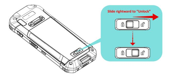
2) Once the battery cover is unlocked, it slightly tilts up and is ready to be removed.
