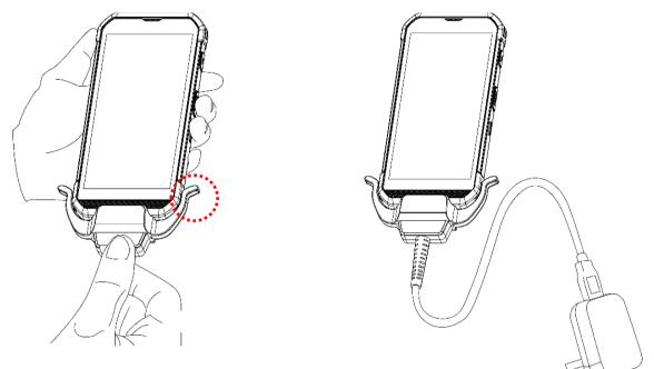
5) Connect the USB plug to the approved adapter for external power connection, or plug it to the USB port of PC/laptop for data transmission/ charging.
