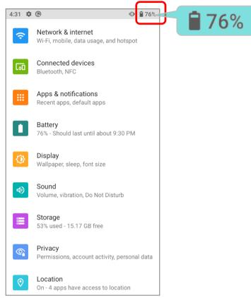
By checking the battery status icon on **Status Bar**, you can tell the battery level remaining in the main battery.
